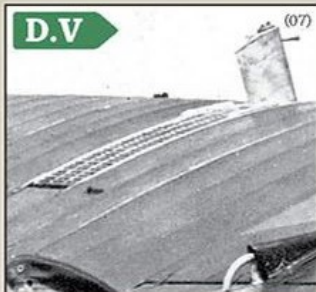
Unpainted aluminium Teves & Braun radiator detail from Manfred von Richthofen's Royal Prussian Jasta 11 Albatros D.V photographed on 6 July 1917.
