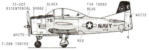
UPPER AIRCRAFT, OUTER WING AND HORIZONTAL STABILIZER- BLUE MIDDLE OF AIRCRAFT, FRONT OF PROP BLADES AND COWLING- WHITE INNER WING- RED AND WHITE STRIPES PROP, BACK AND TIP OF PROP BLADES AND ANTI GLARE PANEL- BLACK
