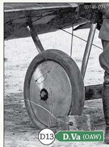
< Undercarriage detail from Albert Dietlin's Royal Prussian Jasta 41 late production Albatros D.V 4612/17 showing the common D.V & Johannisthal built D.Va style of tyre valve access & wheel cover (D14).
