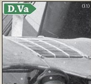
Unpainted aluminium Teves & Braun radiator detail from Robert Ritter von Greim's Royal Bavarian Jasta 34b Albatros D.Va as seen on page 6.
