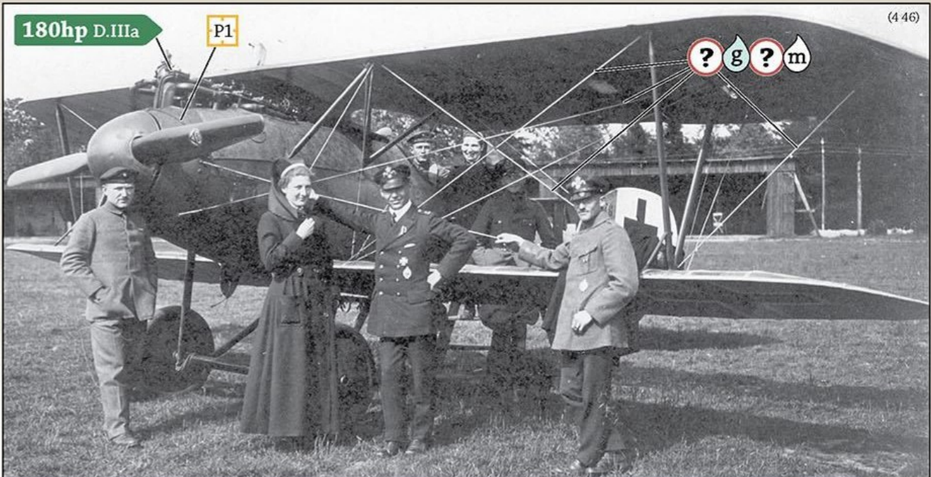
Long serving Johannisthal built Albatros D.Va '76' in service with a Marine Feld Jasta in mid to late 1918. Note the 180hp Daimler-Mercedes D.IIIa engine with water jacketed intake manifold, modified 'post March 1918' balkenkreuz markings and the additional wing strut bracing brackets on the interplane 'V' struts. Also note the mottled camouflage finish on the engine cowlings and the bomb rack fitted under the fuselage for 12.5kg PuW bombs. The very pale rigging wires are unusual and have probably been painted light blue or white.
