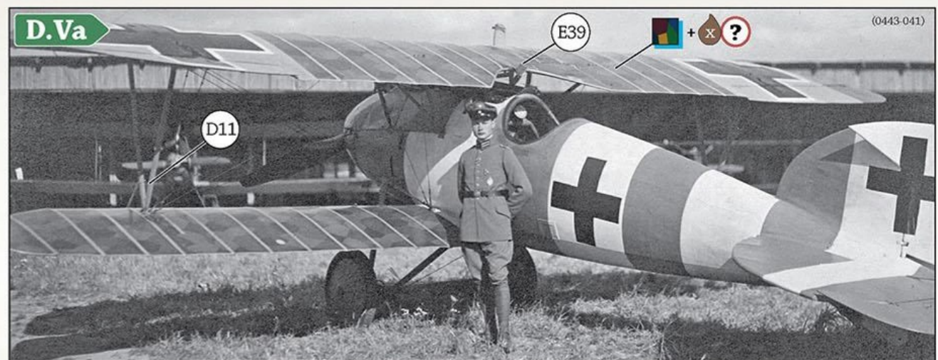
7 victory ace Helmut Dilthey's Royal Saxon Jasta 40 Albatros D.Va features reinforced 'V' strut wing brackets (D11), 5 colour lozenge fabric covering and modified 'post March 1918' balkenkreuz markings. Note the mirror (E39) attached to the top wing cut out.
