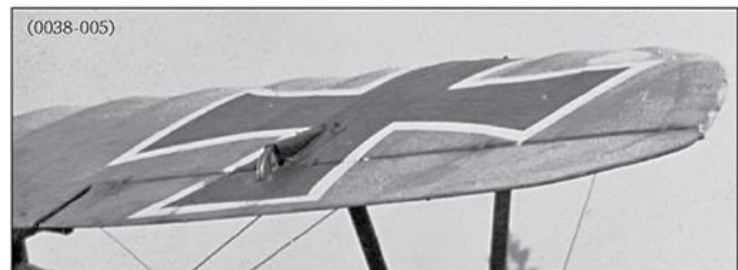
Aileron control horn and cable fairing detail from Karl Schattauer's Royal Bavarian Jasta 16b Albatros D.V
