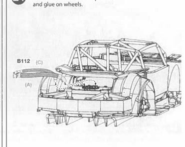
Glue fuel filler into the top of the fuel cell
