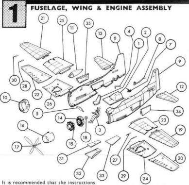
and exploded views are studied before assembly. Note that some parts are best painted before assembly. If stand is to be used cut away wall of plastic from stand in fuselage halves. All parts should be as drawn and moulded tabs adhering to parts should be removed before assembly.
