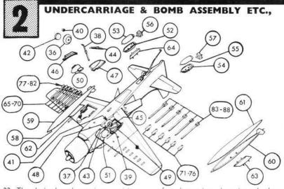
22. The desired undercarriage position should now be selected. For a model with lowered undercarriage, place wheels (36, 37) onto axles at bottom of undercarriage legs (38, 39). DO NOT CEMENT. NOTE: recess in wheels to outside. Place bushes (40, 41) over protruding ends of axles and secure with a drop of cement on ends of axles then cement wheel inserts (42, 43) into wheel
