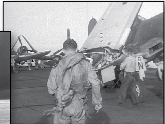
8-N parked aboard Victorious. This view shows the darker wing leading edge and the white gun muzzle cover tape.
