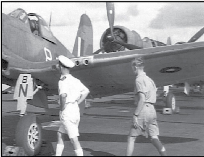
Capt. Denny inspecting 8-N. Note the darker wing leading edge. We believe this was probably due to the leading edge having been waxed to help keep it free of bugs and debris, but we admit we're just not sure!
