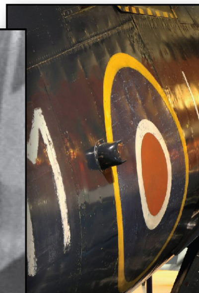
RN Corsairs had a fresh air scoop on either side of the fuselage. These photos show its size and proportions. See profiles for exact placement.
