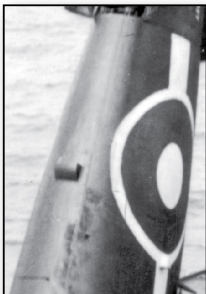
The outlet for the fuselage air scoops was on the belly centerline. This aircraft is nosed-over, providing a clear view of the aft-facing outlet. The tail is toward the top of the photo.
