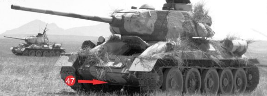
An early exercise with the tanks camouflaged with mud. All the markings have been obscured apart from the bridging class on the lower glacis. Photo:PIO Nicosia
