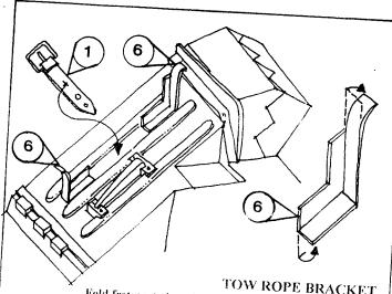
TOW ROPE BRACKET Fold fret parts 6 to shape and locate to kit track guard. Add the retaining strap fret part 1 midway between the brackets.
