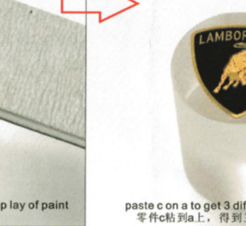
use #800 abrasive file to remove the top lay of paint #800砂棒磨掉上面一层漆
