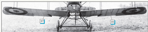
Another view of the undercarriage from DH.2 7851 showing some interesting details such as the compass fairing (A8) under the nacelle, crudely painted cockade (7 & 8) under the port bottom wing which is a replacement upper wing from another DH.2. Note the different style of stencil (35) on this replacement wing.
