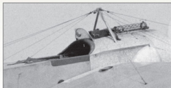
Cockpit coaming detail from Fokker E.III 635/15 showing IMG 08 'Spandau' with internal magazine ammunition feed chute (H1) & (H2), windscreen, compass and shoulder straps of the pilot's 4 point safety harness.
