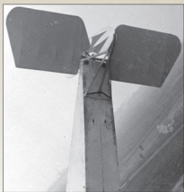
This crashed Fokker, believed to be an E.I, displays the fabric stitching at the rear of the fuselage typical of all Fokker Eindeckers. Note that the fuselage, stitching and elevator control cable outlets have been overpainted with a light colour, possibly light blue, while the elevators remain 'beige' or 'grey'.
