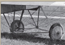
Undercarriage detail from Fokker E.III 635/15 showing strut fairings and rigging details.
