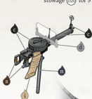
Nacelle detail showing Lewis Mk.II, aluminium nosing, front cowl and external Lewis magazine storage (D20) for 97 round drums (D4).
