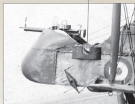
Nacelle detail showing Lewis Mk.II, aluminium nosing, front cowl and external Lewis magazine storage (D20) for 97 round drums (D4).
