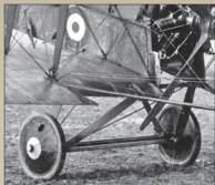
Undercarriage detail from DH.2 7851 showing 32 Sqn C flight wheel markings, axle streamlining (B10), and small metal covered fairing at the rear of the nacelle.
