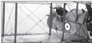
Nacelle and wing detail from DH.2 7851. Note the air intake scoop (A41) pitot tube (B17) and rudder and elevator control cable pulleys (D13) and (D14). The wing struts and pitot tube have been overpainted with the same grey colour.
