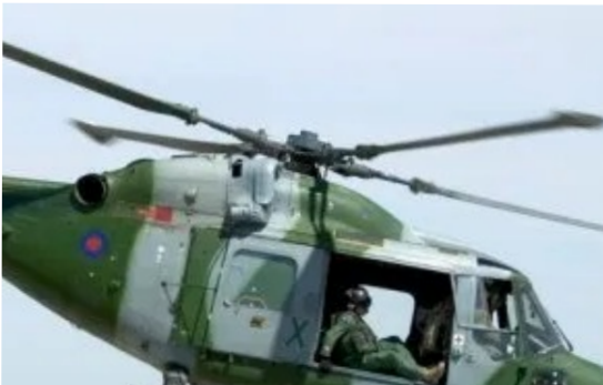
Photo Above & Below: Note standard AH.7 but with particle sand filter intake guards Part no 15/38 and 16/41
