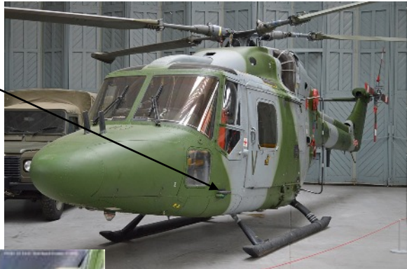
Photo lower right: Shape of lower cockpit window, door handles and small light under step on both sides. Green port and red starboard.
