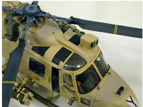
Photo left: Note the two blade aerials just below the cockpit glazing, these are 330mm long and mounted on a small plate 80mm x 150mm. Paint all matt Black. Note shape of lower cockpit window.
