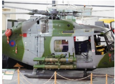
Above: Side view of TOW missile & launcher. Note hand grip aerial behind launcher to the rear of the cabin door. Make this from plastic rod & sprue both sides.
