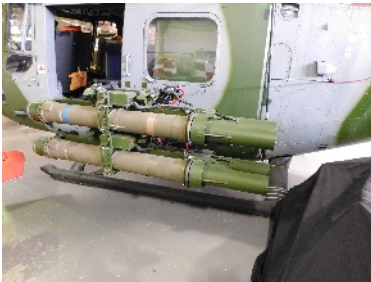
Above: Side view of TOW missile & launcher. Aerial to the rear of cabin door. Armoured seats and cabin door handle.
