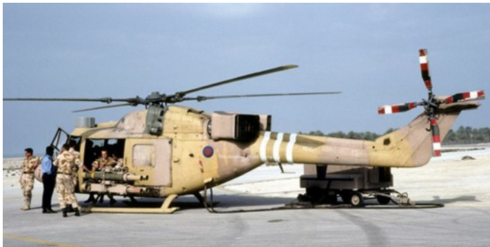
Photo bottom left: Interesting photograph of Lynx AH.1GT XZ221, Showing very worn tail rotor but otherwise the aircraft looks in good condition. Of note is the grey optical sight, no non-slip walkway markings on roof and no handrail type vertical aerials behind the cabin doors. This airframe was converted to Lynx AH.7
