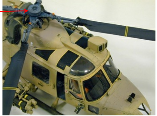
Photo top right: Upper fuselage view of completed model showing the smoke glass cockpit roof window, the optical sight, blade aerials and the walkway markings (although on some aircraft these were painted over as can be seen on the bottom picture) Note main rotor vibration suppressor on top of the main rotor head. Resin part 36. Not all aircraft had this fitted so please check reference.
