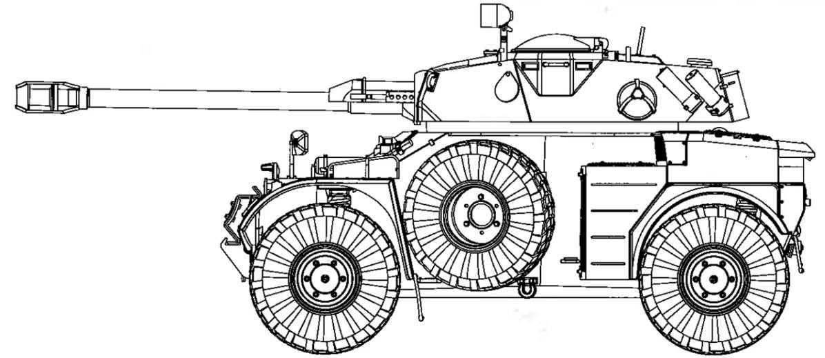
The French Panhard AML (Auto Mitralleuse Légère, or light armored car) is a 5.5 ton lightly armored welded steel 4x4 that first entered service in 1960. With some 4,000 units produced, the AML was developed into multiple specific variants, and was exported widely.
