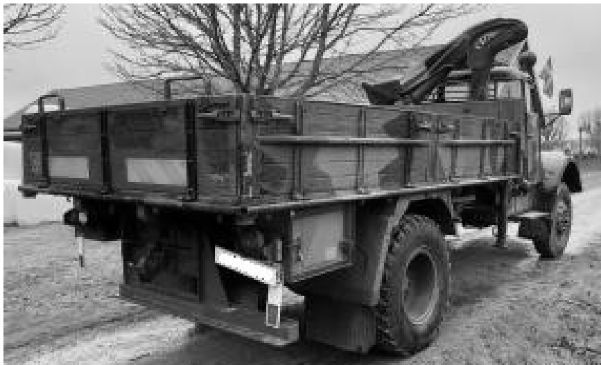
Rear of Ltgb 941B re position of rear frame and lights as well as FOCO Crane
