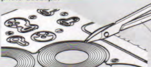
エッチングバサミ Modeling scissors (for photo-etched parts)
