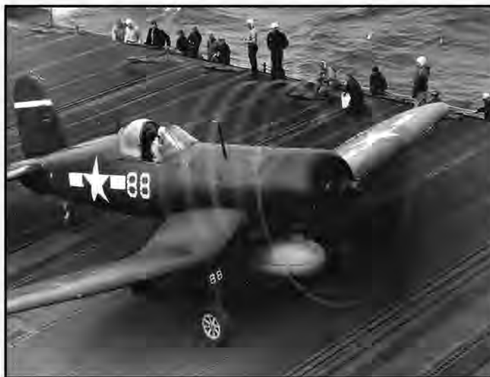
Above: An F4U-1D of CVG-4 launches from the USS Essex in January 1945. The 170-gallon Duramold tank is painted white, a holdover from its previous use on a four-tone camouflaged F4U-1A.
