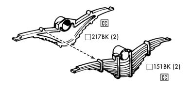
**NOTE:** Cement parts (157 & 156) together. Note there are two pairs of these differentials. Also cement rear leaf springs (151 & 217) together. There are also two sets of springs.
