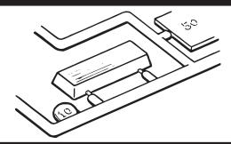
All parts are marked with a number either on the part or on a tab next to the part. Parts should also be carefully compared with the illustration at each construction step.
