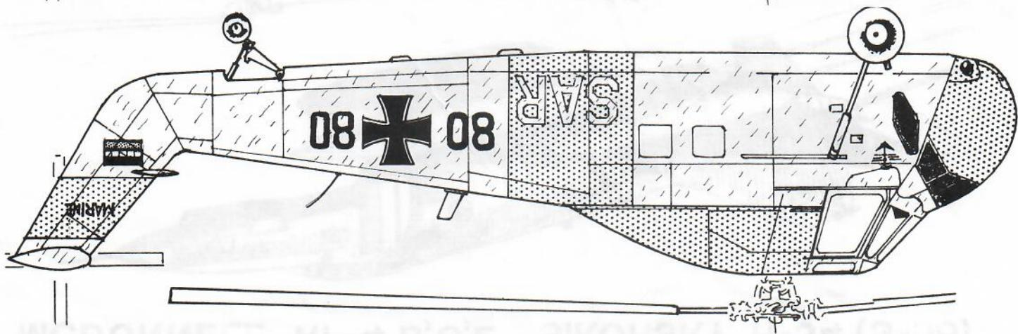
Remove nose with a razor saw. Cut Airmodel nose from sheet and sand edges as required. Glue nose halves together and then to Wessex. Fill and sand as required.
