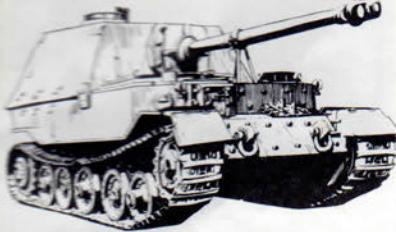
from a rectangular form to a 'T' shape. Because of the chassis alterations, the heavier gun and heavier turret, the weight of the vehicle was increased considerably and the designation was therefore changed to VK 4501 (H). This new projected vehicle had the same main components, transmission, final drive, road wheels, as developed for the VK 3601.
