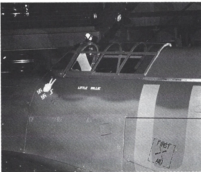
The framework on the windscreen and canopy was painted the same color as the surrounding fuselage. Note the rear view mirror on top of the windscreen. (Detail & Scale photo by Jim Roeder)
