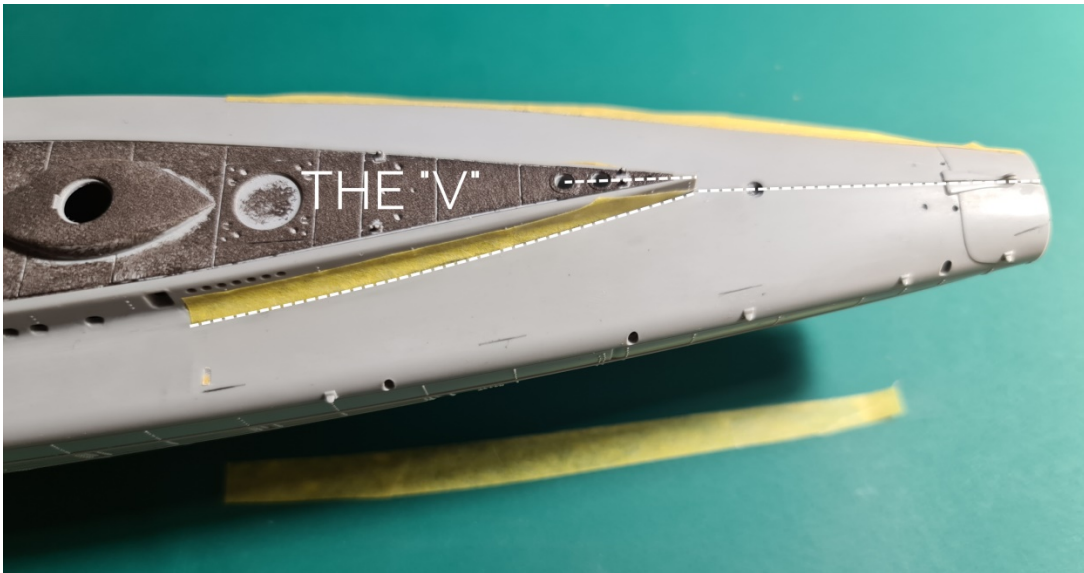
Fig.5.3.) The self-produced tapered masks in place. The Light Grey lines have been painted using a lead pen and THE GUIDE we have created on P.5.1. We'll meet this guy again further below.
