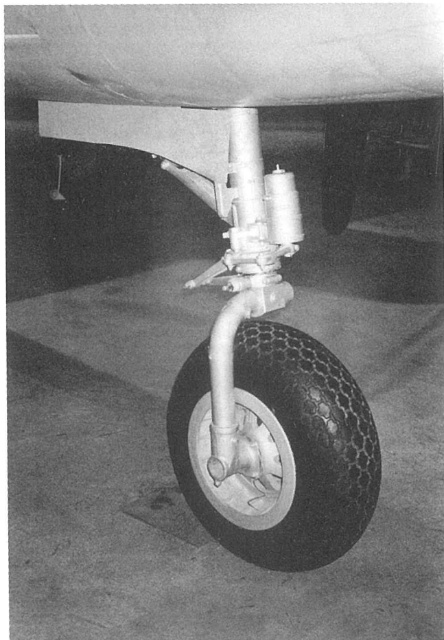
Details of the nose gear can be seen in this photograph. Note the tread on the tire which shows up nicely. The oleo portion of the strut is fully compressed in this view. (Detail & Scale photo by Bert Kinzey)
