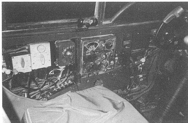
Details of the left side of the cockpit are visible in this photograph. The cockpit wall is flat black, and the switch boxes are also flat black except for the aft two which are flat white. (Detail & Scale photo by Bert Kinzey)
