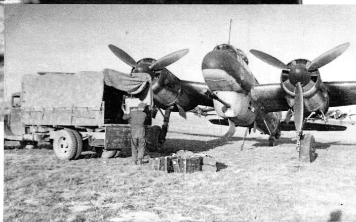
Below: Note additional strengthening of cockpit/nose floor as well as the extra plate behind the normal C-6 gas ejector panel (which is also faired over). Use Tamiya tape to represent these details. Again note the armoured windshield but with MG 81! Note also that the lowest side window (on right side only) as on the A-4 has been re-introduced. (internet photo)
