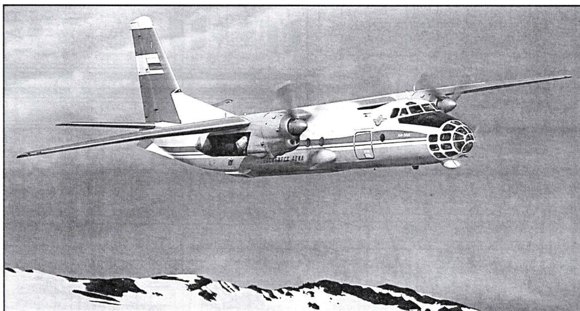
The An-30 was designed by the Antonov OKB in liaison with the Beriev OKB in 1967 for aerial survey and aerial photography. The An-30 is a development of the An-24 and An-26 and is intended for aerial photography and geophysics. The aircraft made its first flight on 21 August 1967. On July 1968 the factory tests were completed. The An-30 was put into serial manufacturing on Kyiv Aviation Plant in 1971. Between 1971 and 1980 115 aircrafts were manufactured and 23 of them were for export.
