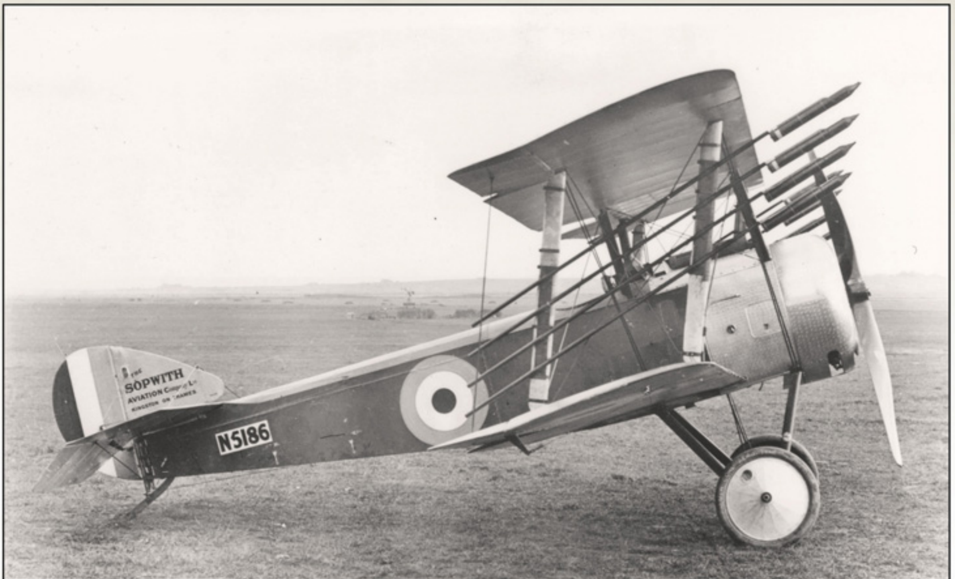
Sopwith built Type 9901 Pup N5186 showing its adjustable tailplane, LePrieur rockets and clear upper wing center section. Most likely pictured here in mid October 1916, N5156 went on to serve in 3,4 and 8 Naval Squadrons before being wrecked in April 1917.
