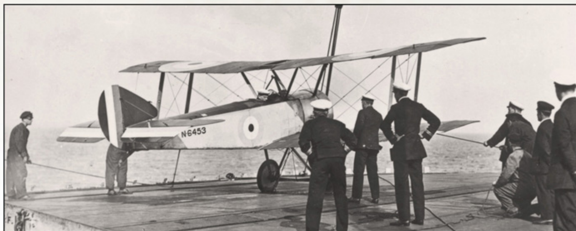
Beardmore built Type 9901a Pup N6453 pictured aboard the aircraft carrier HMS Furious on 27 August 1917. With S/Cdr Busted in the cockpit wearing rather formal headwear, the aircraft firmly (?) tied to the deck and no armament fitted it appears that N6453 is undergoing trials.
