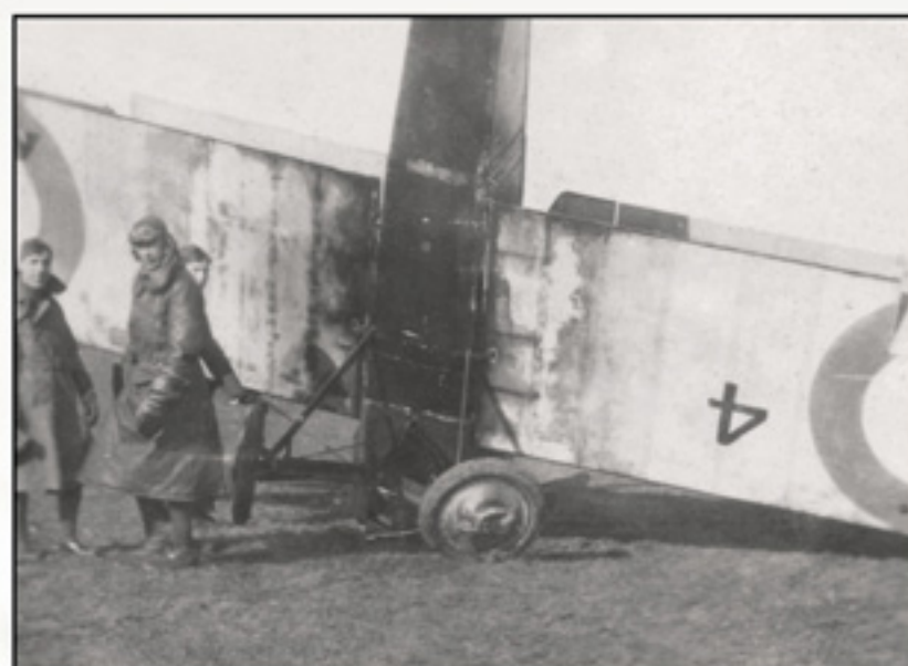
Note the extreme engine exhaust and caster oil staining on the lower sides of this pranged Pup.
