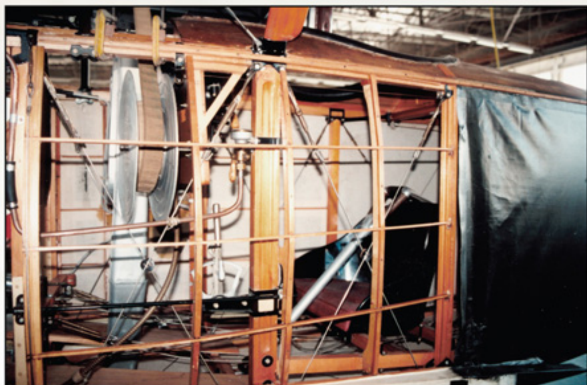
The very accurate Sopwith Pup replica N6160, built by EMK Aeroplanes Ltd/Skysport Engineering from 1978 to 1983, undergoing repairs at the RNZAF museum. Note the various wood tones, CDL fuselage wall interior and the empty belt winder drum for the Vickers Gun. (Photos by David Frowen)
