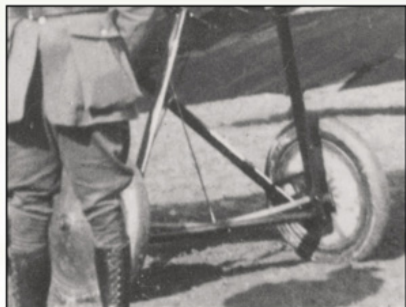
13 Undercarriage detail showing the usual angle of the split axles when absorbing the weight of the aircraft on the ground.
