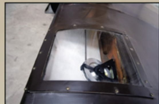
Pulley inspection panel detail from Shuttleworth's Sopwith Pup. (converted from a Sopwith Dove)
