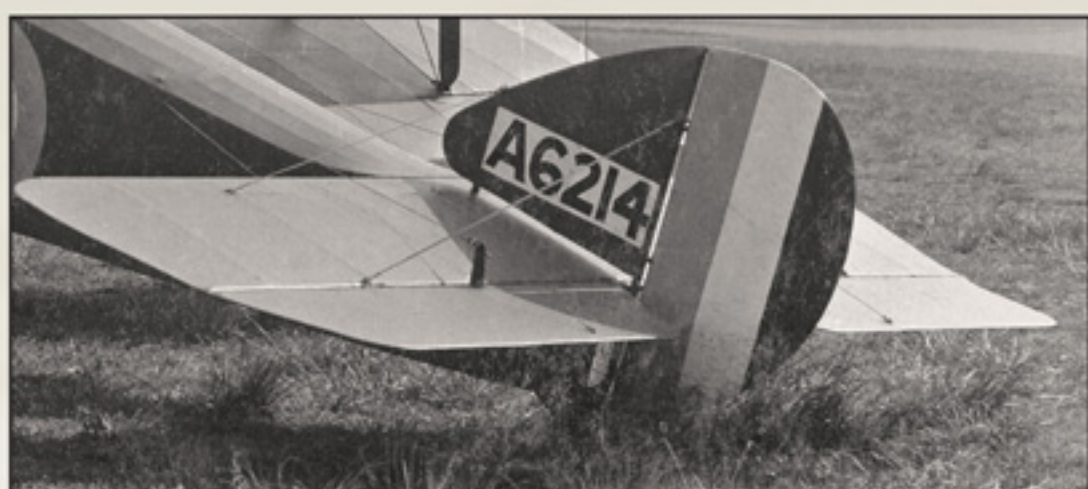
Fixed tailplane detail from Whitehead built Pup A6214.
