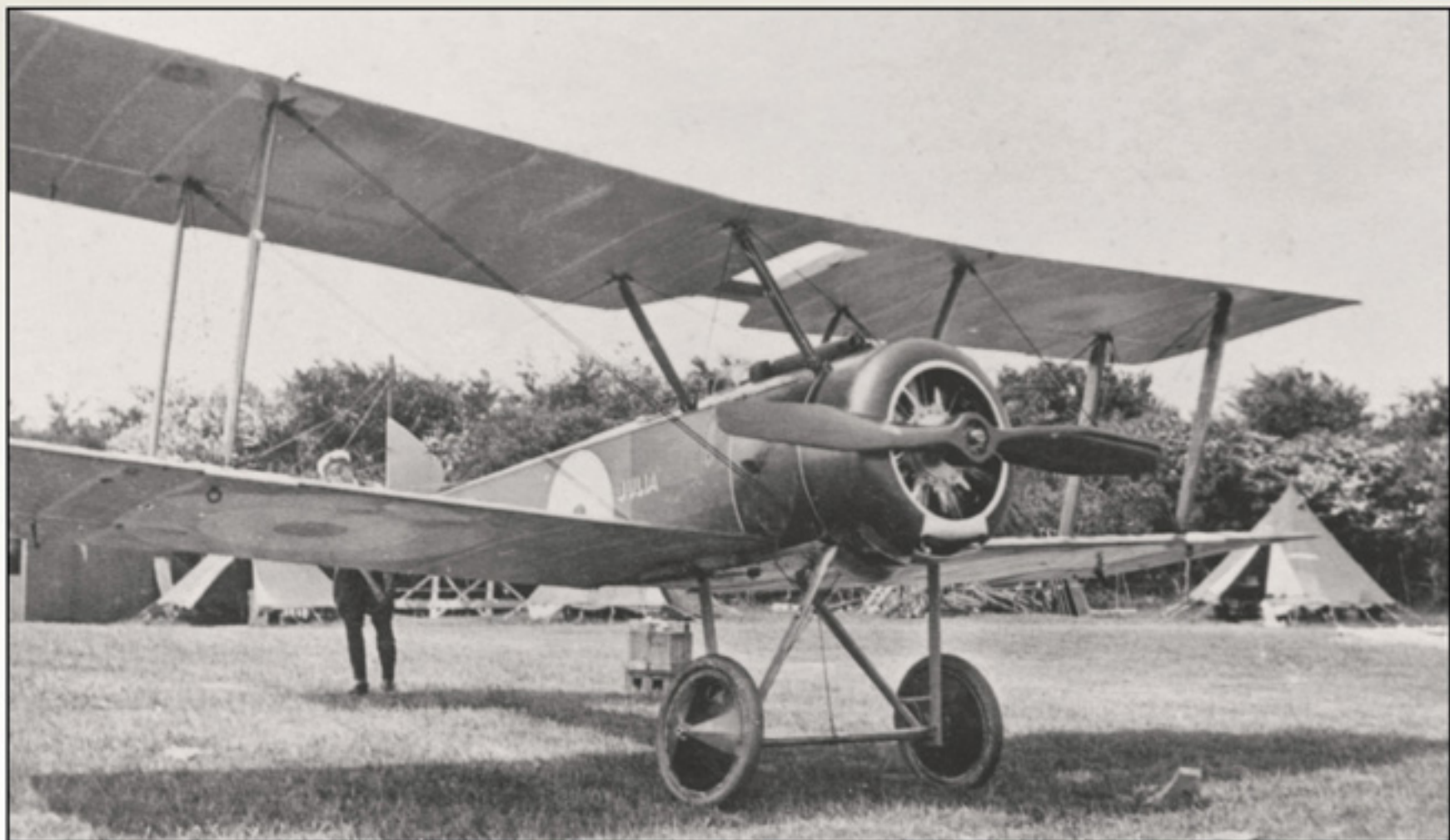
Beardmore built Type 9901a Pup N6442 photographed while on Anti-Gotha duties at the Walmer Defense Flt in June 1917. Note the installation of a Vickers gun for Anti-Gotha duties in place of the Lewis gun more commonly fitted to 9901a Type Pups. Also note the sunlight shining through the white portion of the upper wing cockades indicating that the Proprietary Khaki was painted on afterwards. While this was not an uncommon application process it does not appear to have been adopted universally by all manufacturers.
