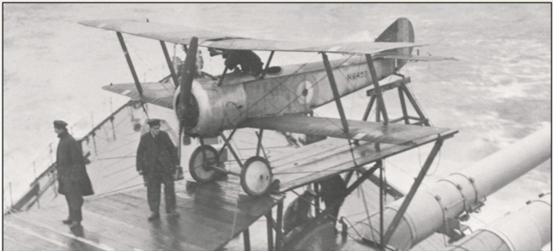
On 1 October 1917 S/Cdr F.J. Rutland successfully flew N6453 off this platform assembled atop B turret of HMS Repulse, thereby proving the concept of shipboard mounted Pups for anti-Zeppelin patrols. The extra stitching visible on the port fuselage side of 9901a Type Pups was to aid access to the flotation bags intended to assist recovery upon ditching in the ocean. Note the heavily weathered appearance of this aircraft after just 2 months service.
