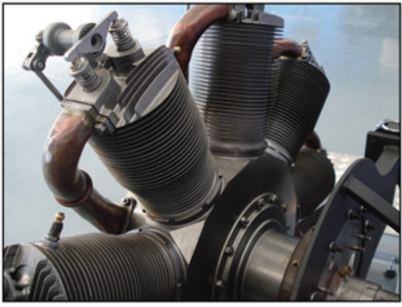
LeRhône 9c 80hp engine. Note the copper intake header assemblies.
