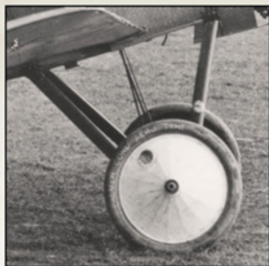
Undercarriage details from Sopwith built pup N5186. Note tyre marking and manufacturers logo decal on front undercarriage leg.
