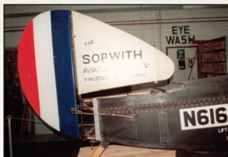
Sopwith Pup replica N6160 displays the general arrangement of its fixed tail plane fittings. (Photo by David Frowen)
