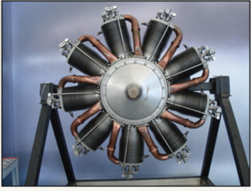
LeRhône 9c 80hp engine. Note the copper intake header assemblies.
