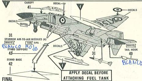
Cement (4) Parts 31 into place on the underside of Fuselage. Apply Bottom Wing Decal and let dry before attaching Assemblies 4. Cement (2) Assemblies 4 into place as shown. Now, cement Part 40 to the rear of the model in either the UP or DOWN position. Carefully, cement Part 41 to the Cockpit area. Cement Part 43 into Part 42 and let dry thoroughly. Place, or cement model down onto Part 43. See the 3-View Drawing on the opposite side of sheet for further Painting Suggestions and Decal placement.
