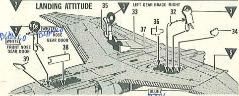
Turn model upside down and cement the Right Main Gear into Assembly 5. Next, cement Parts 32, 34 and 36 into place. Repeat the same procedure for the Left Main Gear using Parts 33, 35 and 37. Now, cement the Nose Gear into place and cement Parts 38 and 39 into place.
