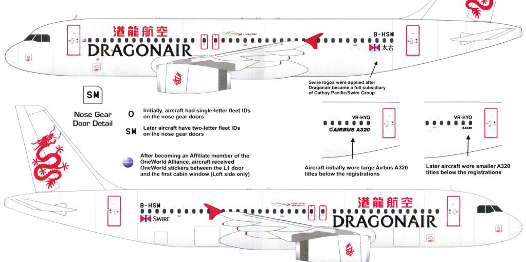
We strongly urge you to fill in the kit's open windows! Wings and horizontal stabs have standard bare metal leading edges, always consult prototype photos.
