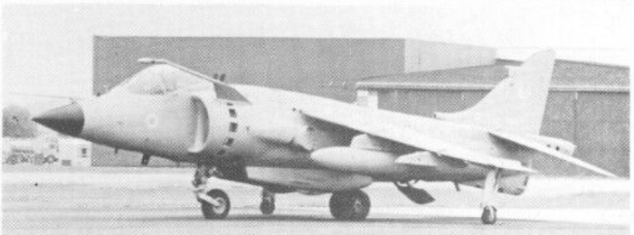
6. Sea Harrier FRS1 XZ499 (later coded '99' of Hermes Air Group) departs Yeovilton 30 April 1982 to join the Task Force. This was one of the few occasions when Sea Harriers have been seen fitted with IFR probes, though note that ferry wingtips were not fitted. This scheme existed until shortly after 809 Sqn machines joined the two carriers. Photo: G. Long. © MODELDECAL 1983
