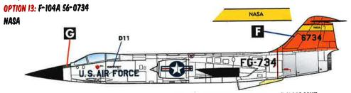
THIS MASA TEST JET HAS SOME INTERESTING MODIFICATIONS. NOTE RELOCATED PITOT TUBE AND OLIVE DRAB ANTI GLARE PANEL.
