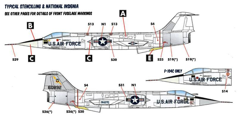
(\*): DECALS "SI9" AND "S26" WERE MISTAKENLY PRINTED AS A SINGLE DECAL - PLEASE CUT THESE MARKINGS VERTICALLY IN THE MIDDLE TO OBTAIN TWO SETS OF EACH, AND APPLY AS SHOWN.
