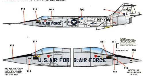
NOTE NF-104 SPECIFIC STENCILLING ON THE NOSE (TIO, TII, TI2) AND THE DECALS TO REPRESENT THE THRUST PORTS (TI8).
