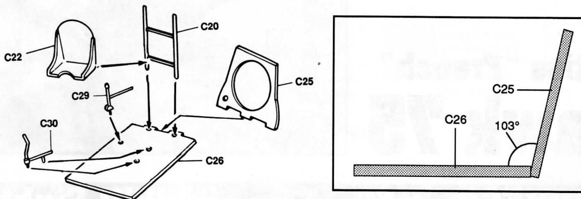
**2****Fuselage Assembly / Assemblage du Fuselage**
