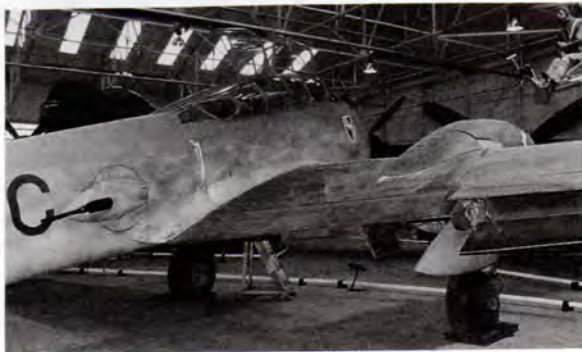
This photograph shows where the right wing joins the fuselage. The joint is rounded and smooth.
