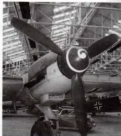
The complete left engine nacelle is shown here. Note the radiator under the nacelle and the exhaust along the side.
