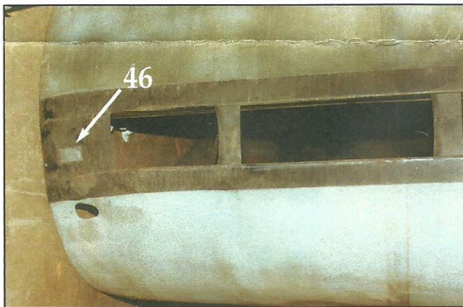
Port side of engine cowling showing correct positioning of data plate, decal #46.
