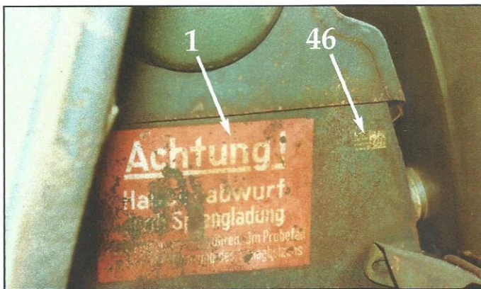
Data plate on armored head rest, decal #46. A portion of one of the six desiccant tablets in the canopy can be seen just to the right of the armor plate. 'Achtung' decal #1.
