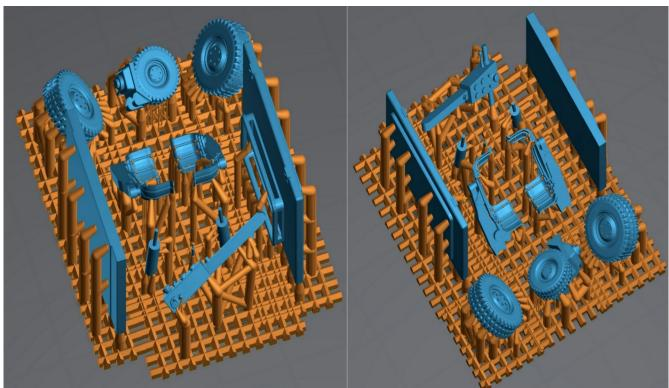
To remove the supports, you can use a sharp blade or nippers. To glue the different pieces, use cyanoacrylate-based glues.
