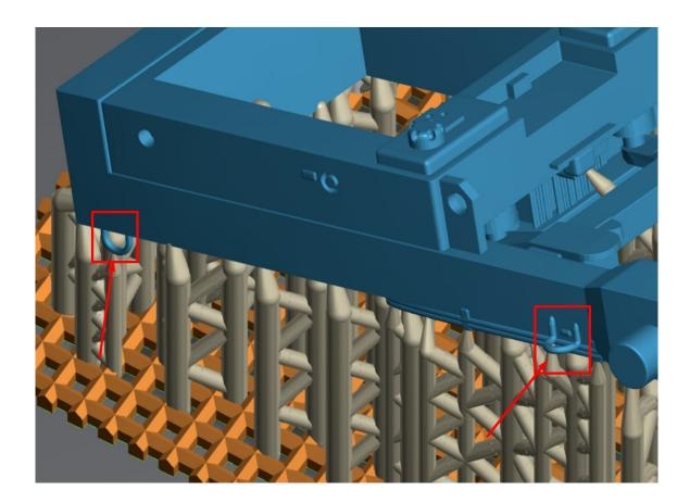
**Tip** → Start cutting supports from the base; this will make it more challenging to break fragile details.
