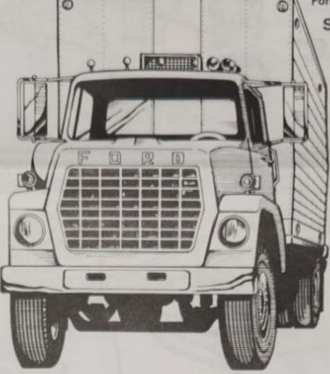
was designed to tilt forward for engine access.
