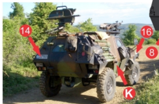
After 2005 tyre pressure markings were added in at least two versions. Also tactical sign holders were added to the front doors.
