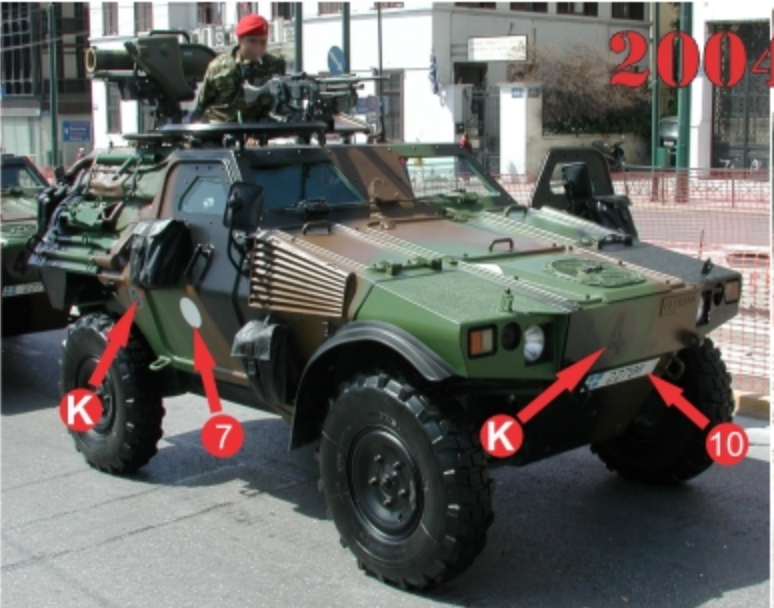
After 2005 tyre pressure markings were added in at least two versions. Also tactical sign holders were added to the front doors.
