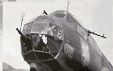
Field modified nose glazing with forward firing MG FF. MG-15 in A-Stand (mounted in the windshield). Note a non-standard MG 15 pointing to the side.
