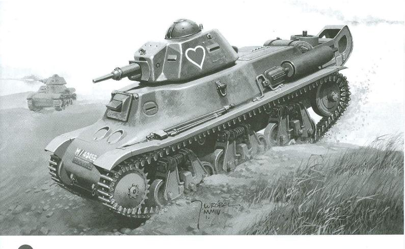
The Hotchkiss H39 was re-designed from her family H tank series for the French Army Cavalry tank in 1938~39. The H39 was armed with the longer L/33 gun and 120PS motor. Large number of this tank fell to German hand in 1940 invasion. Many of these H tank, after modification were issued to German units from 1941.
