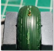
From the interior part of the wheel, drill a 2mm hole to insert the piston. Drill a little bit with a round driller if needed.
