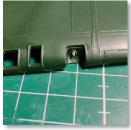
For the landing lights, drill a 1,2-1,4mm to pass the head of the LED Secure it with the UV glue. Tape the LED wire.
