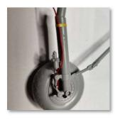
From the pistons, you can fix the electric wire along the landing gear, as if it was a hydraulic pipe.
