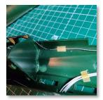
The cockpit illumination is done by placing a LED on the 'ceiling' of the cockpit. The cable will pass from the front to the back, hiding it as much as possible.
