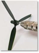
Cut the excess shaft 3D part, so that only the interior of the shaft will remain.
