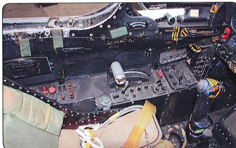
Typical Mirage 5BA cockpit layout with all black cockpit tub, side walls and seat. Seat cushion in Khaki. (Photos AirDOC)
