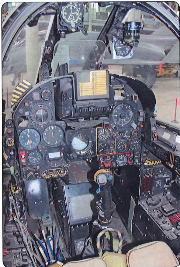
Typical Mirage 5BA cockpit layout with all black cockpit tub, side walls and seat. Seat cushion in Khaki. (Photos AirDOC)
