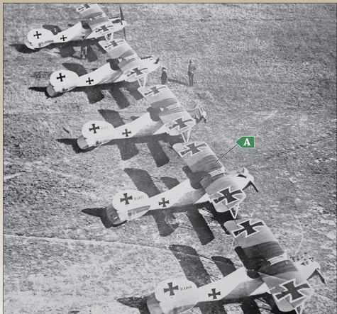
A line up of brand new Albatros D.V from the 1st production order including 1166/17, 1177/17 A and 1178/18. Note the variations in wing and tailplane camouflage colour placement.
