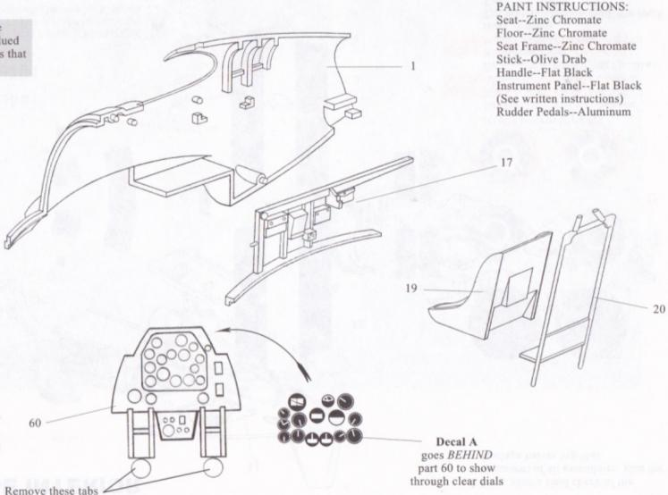
STEP 2-FUSELAGE INTERIOR ▲ Glue the radios into the right fuselage half. Place the part against the back of the forward
