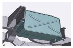
Fuel tank, join halves together. **L** brackets locate onto outriggers as shown.
