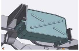
Fuel tank, join halves together. **L** brackets locate onto outriggers as shown.
