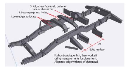
Fit cross braces and outriggers to complete chassis.
