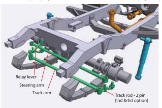
For Ihd swap location for 2 pin track rod and relay lever to the opposite hub A dedicated lhd part is supplied, rotate steering arm through 180 deg.
