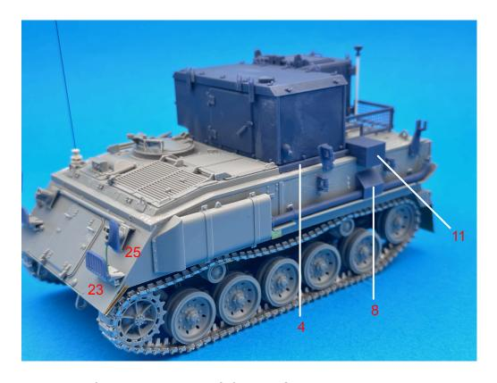
Parts 24 & 25 are handed Left & Right Clean out holes with 0.4mm drill and join to 22 & 23 with brass rod
