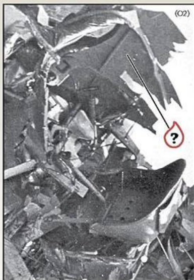
The sad wreckage of Royal Bavarian Jasta 34b Pfalz D.IIIa 8023/17. Note the darker tone of the fuselage interior and that the brackets on the instrument panel appear to be painted black while the ammunition magazines are unpainted aluminium. The seat appears to have a pouch of some sort fixed to its rear and is missing its cushion.
