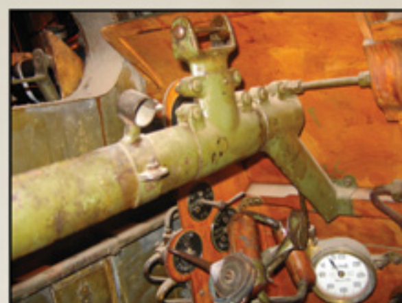
Close up of the LMG08/15 mount showing the empty bracket for the tachometer. Note also the various switches on the instrument board.
