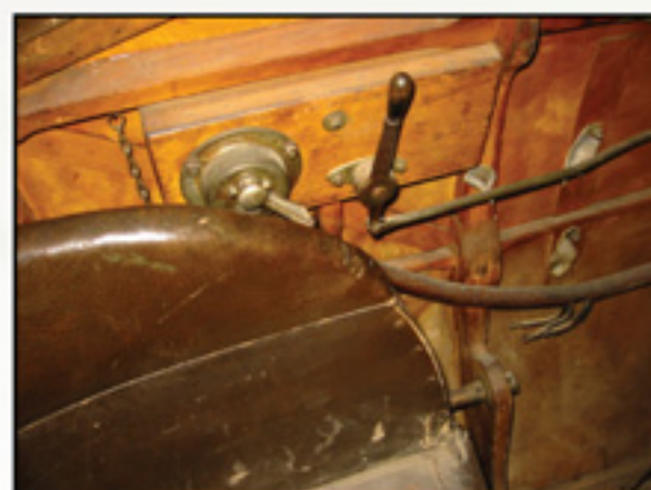
Throttle and Bosch engine switch. The switch (key) of the Bosch switch is attached to the small chain just visible. You can often see these keys hanging from this chain outside the cockpit in archive photos when the engine is not about to be started.
