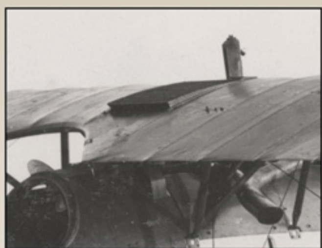
Daimler-Mercedes radiator detail from Albatros D.Va D.5390/17 shortly after capture.
