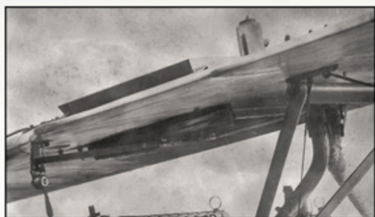
Daimler-Mercedes radiator detail from an unidentified D.Va showing a second style of shutter control lever. Note that the front water pipe from the radiator is wrapped in white asbestos cloth for insulation.
