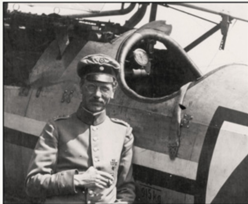
Note the trimmed windshield and safety harness strap hanging from the cockpit of Von Hunoldstein's Jasta 14 Albatros D.Va.
