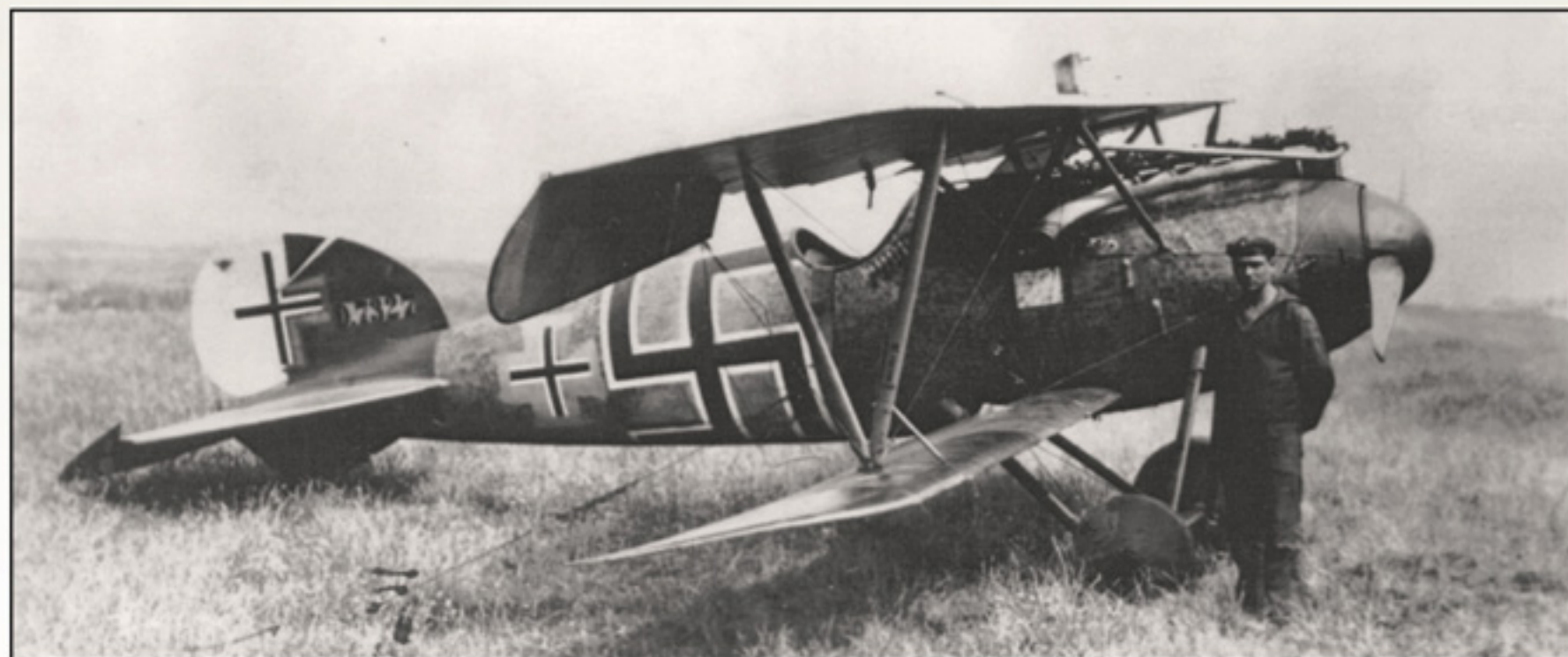
Lothar Weiland was forced to land his Seefrontstaffel 1 Albatros D.Va D.7327 after being shot in the left ankle during combat with Sopwith Camels of 213 Sqn on 30 July 1918. As a result of his injuries he would lose his left leg. The fuselage and cowling have been heavily mottled with dark green paint most likely applied with a 'loofa' type sponge. Previous versions of the national markings have been painted out with grey paint, most likely simply mixed from the white and black paint supplied to convert the crosses. The Orthographic film has caused the chrome yellow unit markings of the tail plane and spinner to appear dark in this photo.
