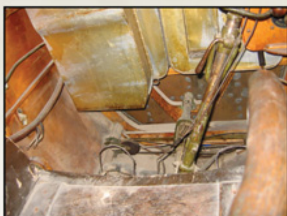
Aileron control cable pulley detail.
