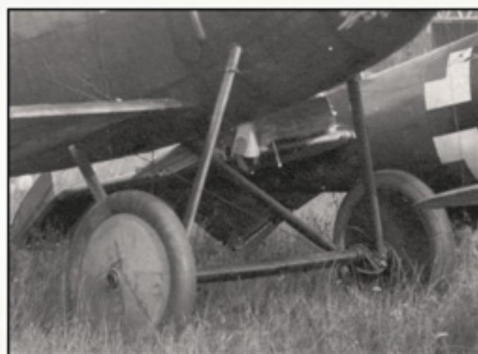
Undercarriage detail from von Hippel's Albatros D.Va D.7353/17.
