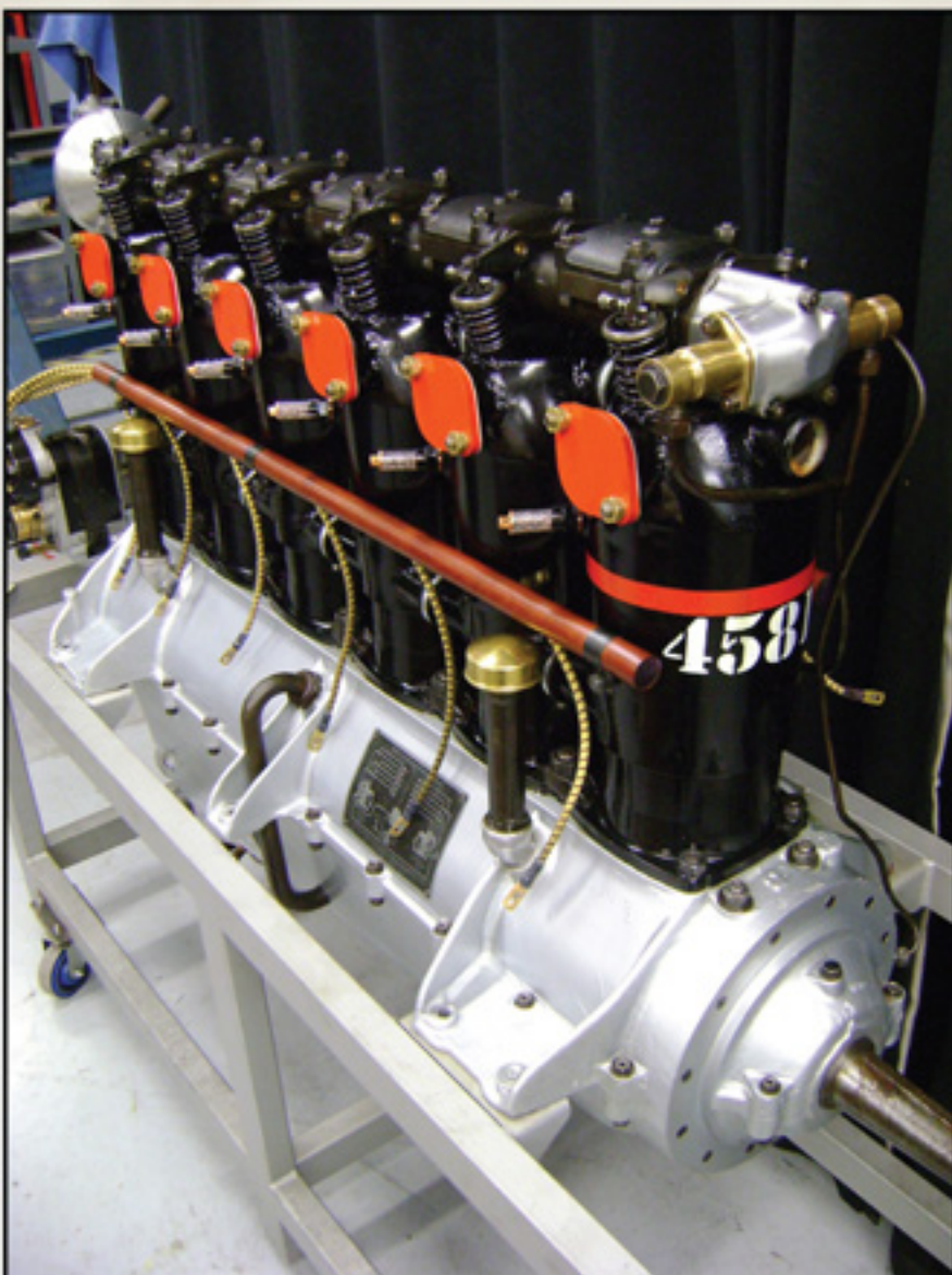
The serial number of the engine was often stenciled on the front cylinder, but not always as can be seen in our photo on page 7. The red band signifies an over compressed cylinder. In period photos it is very difficult to distinguish a red band against a black cylinder.
