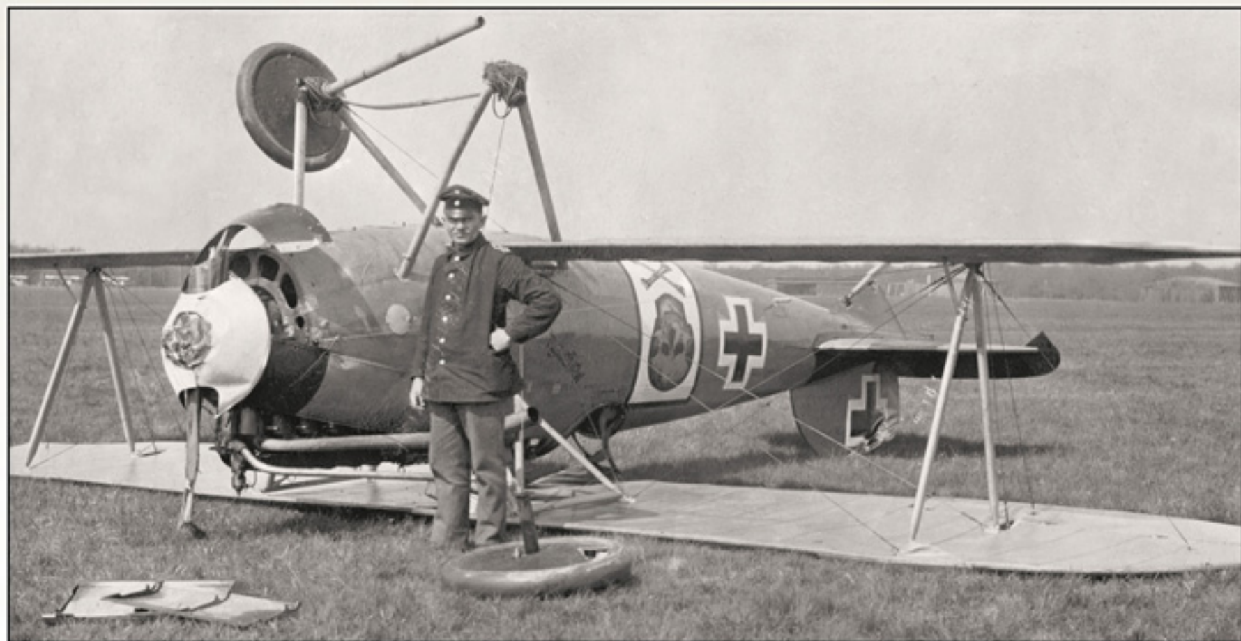
A mechanic poses in front of Hans von Goessel's crashed OAW built Albatros D.Va, the two undercarriage axle wing fairings at the bottom left of the photo possibly indicating the start of his salvage mission. Note the aileron control wires entering the upper wing, undercarriage bungee cords and OAW style lifting handle 'bar' protruding from the rear side of the fuselage. The name under the cockpit opening reads 'Margarethe'.
