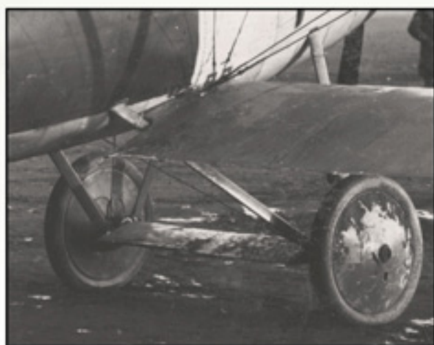
Undercarriage detail from Albatros D.Va D.5390/17 shortly after capture. Note the hinge detail on the leading edge of the axle wing, the canvas covers protecting the bungee shock cord and the chipped and weathered nature of the metal spoke covers.
