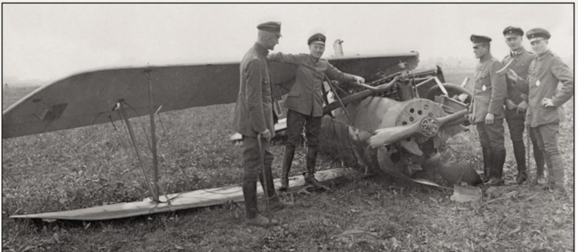
The apparent levity of the attendant pilots indicate that this Albatros D.Va crash landing probably wasn't fatal. The repair patch under the right wing tip appears very similar to that shown in the photo of D.Va D.7353/17 on page 21, perhaps it is the same aircraft? The shattered backing plate to the spinner appears to be made from plywood instead of pressed aluminium in this instance. The pilot at far right is holding the remains of the tail skid!
