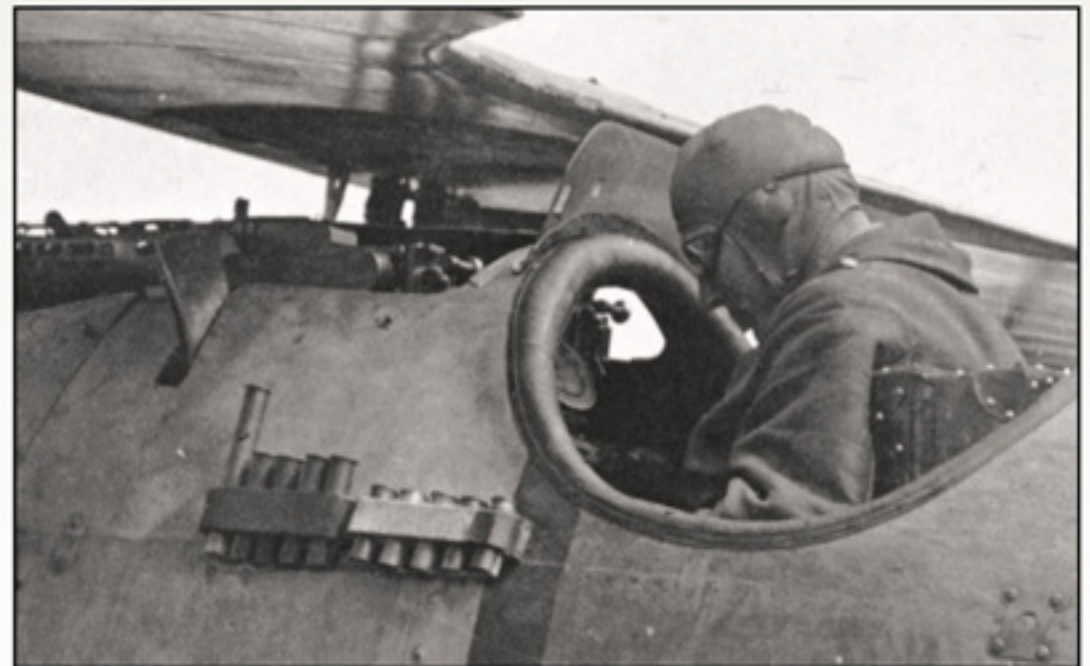
Note the flare racks and what appears to be some sort of medieval torture device the unidentified pilot of this Albatros D.Va is using as a seat back cushion. Also note the 'peep holes' cut into the windscreen for sighting the guns.
