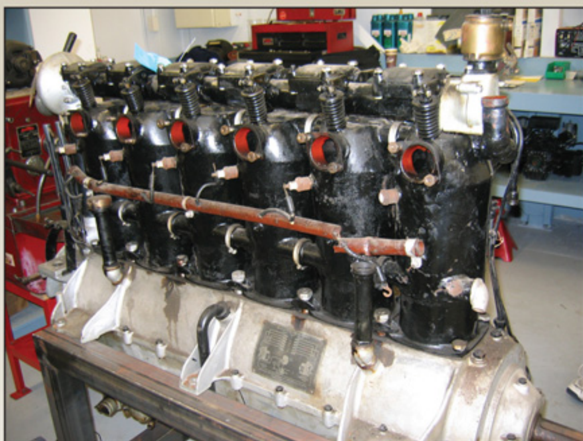
Right side of the engine. Note the newer location of the water pipe running through the cylinders and the position of the data plate.
