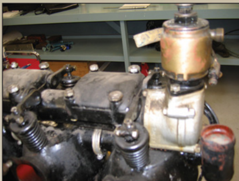
Large air pump (E29) characteristic of the 180ps Daimler Mercedes D.IIIa. Note the rocker boxes (E27) are now positioned to the rear of the springs.
