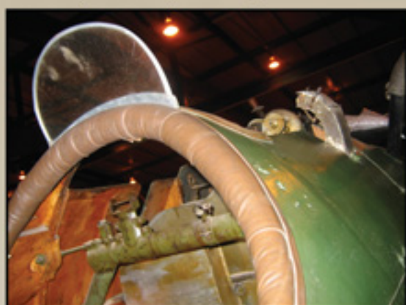
Cockpit padding and LMG 08/15 ammo chute detail.
