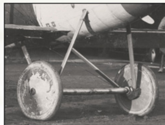
Undercarriage detail from Albatros D.Va D.5390/17 shortly after capture. Note the hinge detail on the leading edge of the axle wing, the canvas covers protecting the bungee shock cord and the chipped and weathered nature of the metal spoke covers.
