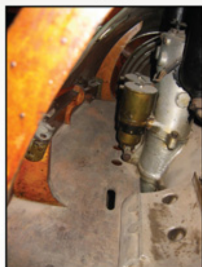
Left engine bearer. Note the engine shown here is a very late model Daimler-Mercedes D.IIIau featuring a generator mount that is not applicable for the D.V.
