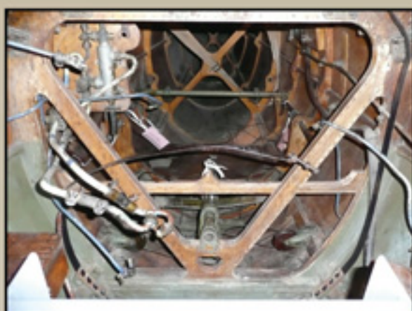
Looking towards the rear from inside the engine bay we can see the D.Va aileron control cable pulleys. (via Colin Owers)
