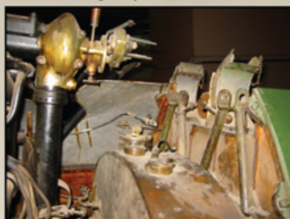
The rear of the engine, top of the fuel tank and front mounts for the LMG 08/15 machine guns.
