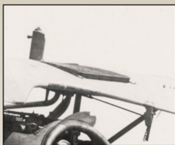
Daimler-Mercedes radiator detail from von Hunoldstein's Jasta 14 Albatros D.Va. Note the shutter control lever at right.
