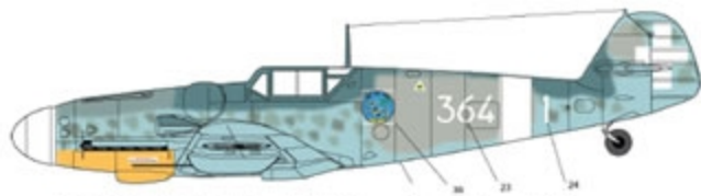
BF 109G-6/R6 W.Nr. 18391. 364 a Squadriglia, 150 o Gruppo Autonomo, Sciacca, July 1943. Aircraft likely to have been flown by Cap. Mario Bellagambi. 74/75/76 camouflage with 02/70 mottling. German markings oversprayed in possibly Grigio Azzuro Chiaro. Wing insignia applied.
