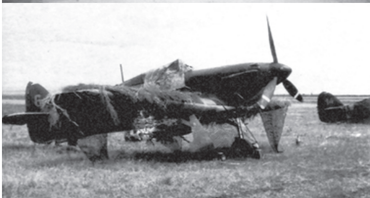
The burned wreck of Hurricane "15" lost on Saltz airfield. Clearly visible the fabric covered wings, typical for Yugoslav-built Hurricanes.
