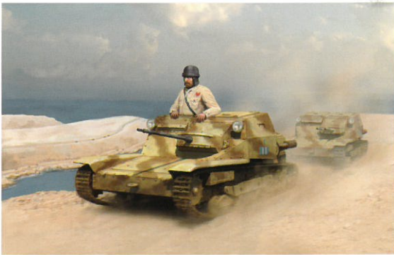
Carro Armato L35/c ( C.V.33/II Serie ) fitted with the Swiss "Solothurn" S18-1100 20mm anti-tank gun
